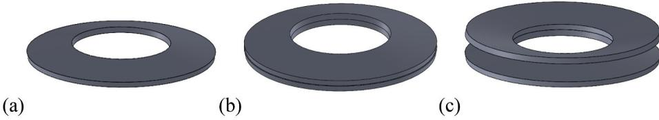
**Figure 5.** Disc spring: (a) basic form; (b) stacked in parallel; (c) stacked in series.
